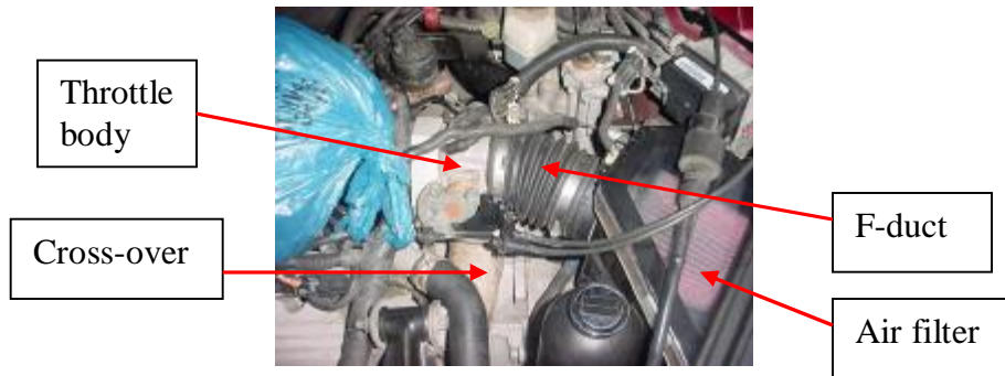
Fig 7: Throttle body and F-duct in the visible spectrum
